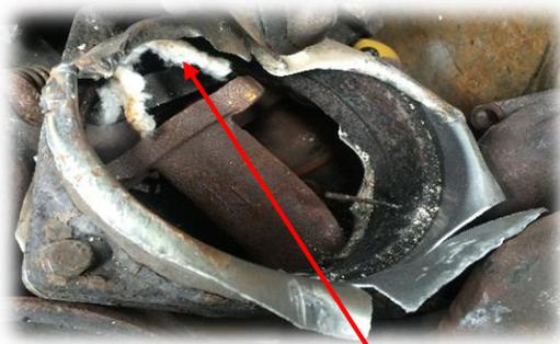
RCF attached to the casing but not held with banding.
