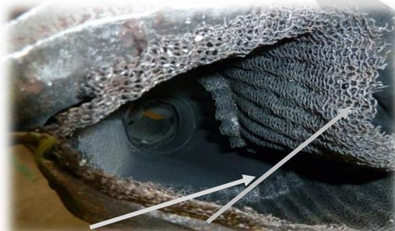
Metal mesh matting in a catalytic converter with no RCF matting
